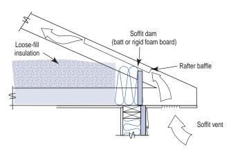
This oversized truss shows loose-fill insulation that is blocked or dammed at the eave with a soffit dam (a piece of fiberglass batt or rigid insulation). A rafter baffle creates a channel for air flow.
