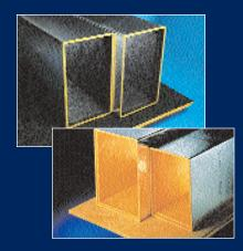
Fibrous glass ducts are fabricated from 1", 11/2", or 2" thick boards of insulation material manufactured from resin bonded inorganic glass fibers. The outside surface of the board is a factory-applied reinforced aluminum air barrier and water vapor retarder. Fibrous glass duct systems can be easily fabricated, either in the contractor's shop or at the job-site, and eliminate the extra fabrication steps required when applying thermal and/or acoustical insulation to sheet metal ducts.
