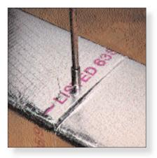
During fabrication and installation, unintentional mishaps such as a dropped tool can occur and the duct must be able to withstand them. Even in routine service, air ducts may encounter abuse. This test indicates just how well the duct will resist damage during and after installation.
