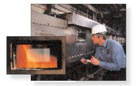
Test Procedure: The UL Surface Burning Characteristics test, recognized as a standard test for evaluating all types of building materials as to their performance when exposed to heat and flame, is conducted in a 25-foot tunnel, with fibrous glass duct – including closure system forming the ceiling. When a gas flame impinges on the duct material, it must not exceed a flame spread rating of 25. Smoke developed must not exceed a rating of 50.
