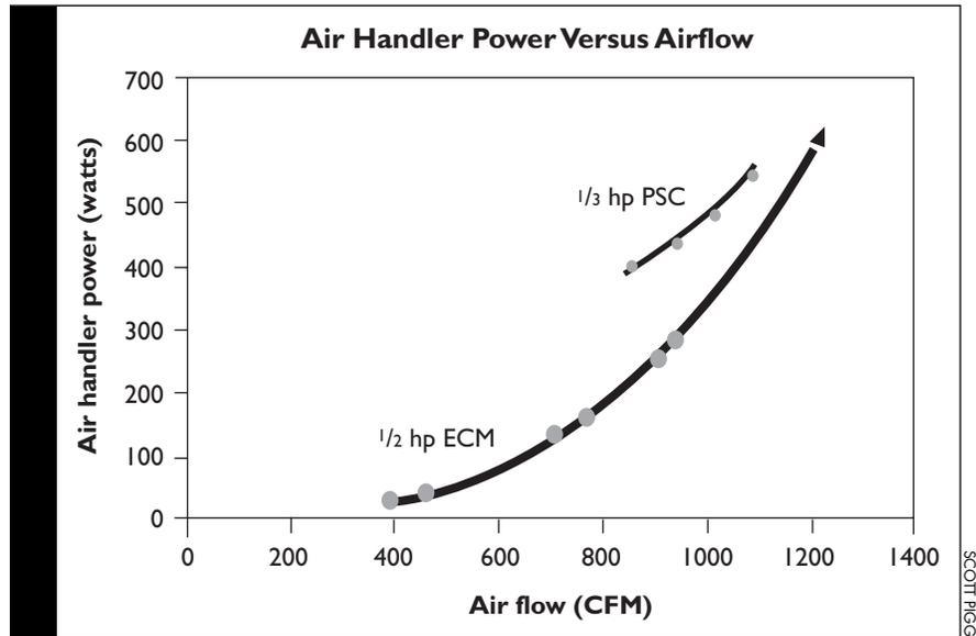
**Figure 1.** The air flow range of the furnace with the ECM extends beyond that shown in the figure, but the furnace powered by the PSC motor is limited to the four speeds shown. The two 60,000 Btu/hr furnaces operated in similar static pressure environments.
