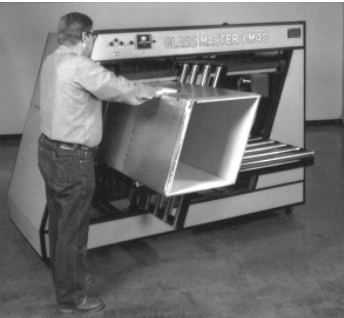
Fig. 12. Fibrous glass duct closure machine
