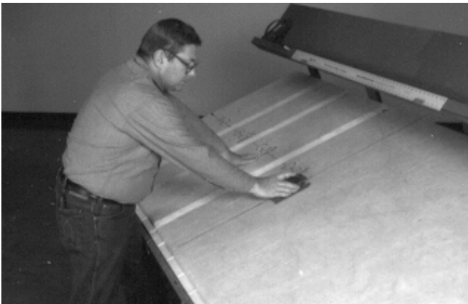
Fig. 10. Hand grooving fibrous glass duct board
