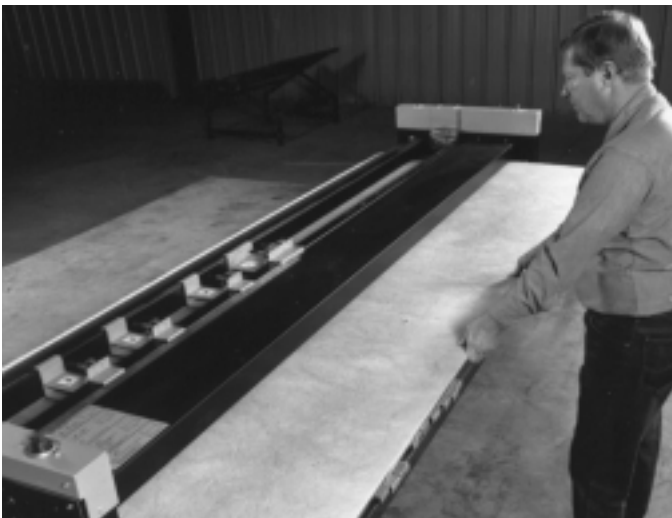
Fig. 11. Machine grooving fibrous glass duct board
