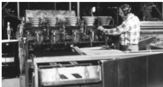
Fig. 15. Shop fabricating with fibrous glass duct liner
