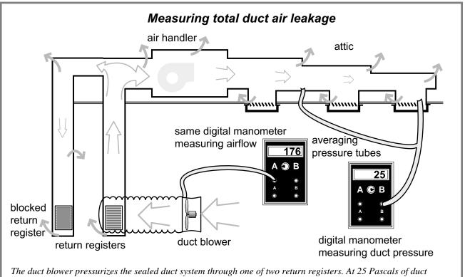
pressure, these ducts have 176  $CFM_{25}$  of duct air leakage.
