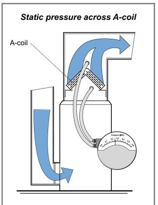
Measuring this static-pressure difference can estimate airflow and detect dirt, especially if manufacturer's graphs or tables are available.
