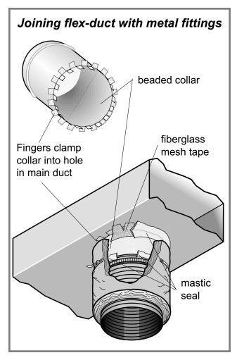
of hand-applying sealant to seams, among others, can save 10 percent in existing homes and 15 percent for new homes.<sup>3</sup> If duct leakage is reduced, cooling and heating equipment can be downsized for additional savings. Reducing leakage can also increase cooling and heating output at registers. Savings are greater for new than for existing installations because retrofitters do not have full access to duct, plenum, and boot joints.
