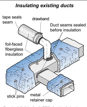
Exterior foil-skrim-kraft (FEK) duct insulation is attached to existing metal ducts with stick pins or drawbands. FSK tape is used to seal seams in the insulation.
