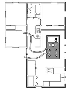
The bedroom, with reference to outdoors, measures 8 Pascals, indicating a pressurized bedroom, due to imbalanced airflow. Unbalanced airflow in a singlereturn system separates the home into pressurized zones, promoting air leakage through the building shell. reference pressure location.
