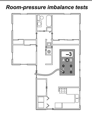
The main body of the home, where the single return is located, is depressurized with reference to outdoors. The main return and closed interior doors cause this unwanted pressure difference.
