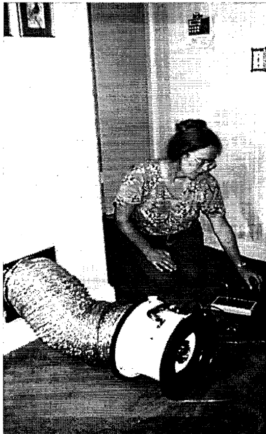
Figure 5 Alternative Duct Blower attachment using a large register.
