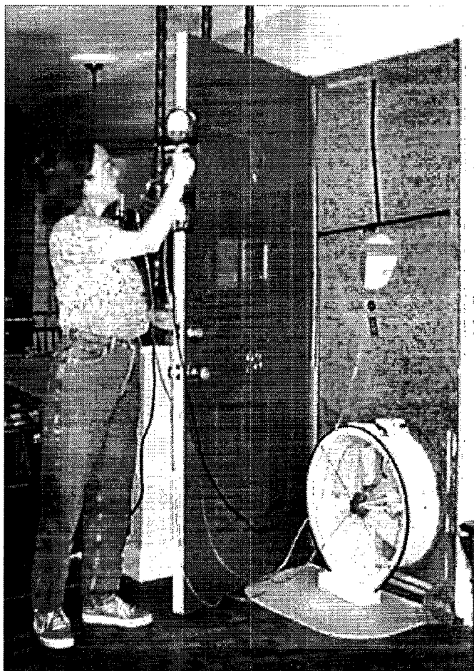
Figure 3 Blower Door mounted in entryway of home in use during duct leakage evaluation tests.
