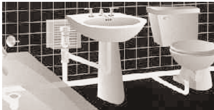
AIR ADMITTANCE VALVE BEHIND SINK
