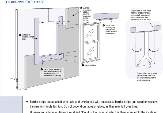
Housewrap technique utilizes a modified "I"-cut in the material, which is then wrapped to the inside of the window frame and fastened. The head flashing and barrier strip are fastened and "shingled" under a flap that is cut in the wrap. These seams are then taped.
